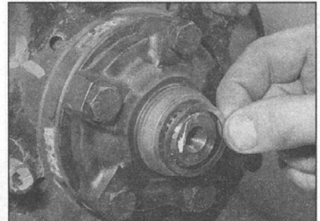
3.10b . . . and recover the thrustwasher(s)
