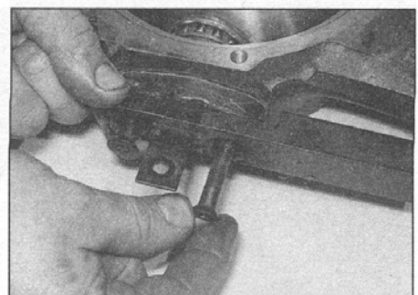
6.9 Remove the lower swivel pin retaining bolts and recover the mudshield bracket, noting which way around it is fitted
