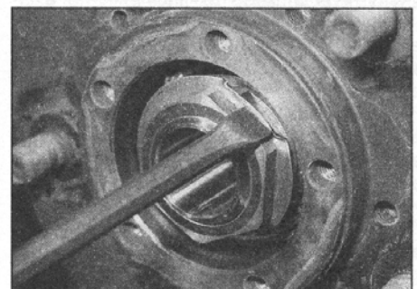
9.3 Bend back the lockwasher from the locknut's flat using a suitable chisel
